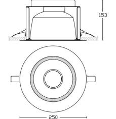
Cut out diameter range: 210 / 230 mm Weight: 1.0Kg Weight excludes driver
