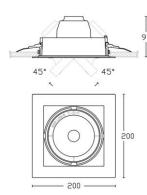
CUT OUT SIZE 177mm x 177mm Weight: 1.1kg MAX excluding drivers All dimensions in mm
