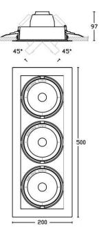
CUT OUT SIZE 177mm x 455mm Weight: 3.0kg MAX excluding drivers All dimensions in mm
