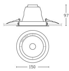
Cut out Ø 140mm Weight 1.0 – 1.5kg All dimensions in mm
